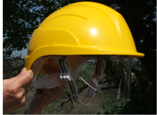
CENTURION HELMET: Built in eye protection. reduced peak. Extra neck protection. Sewn terylene cradle-adjustable from 51 to 63cm.
